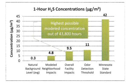
Odors from asphalt facilities are primarily composed of hydrogen sulfide (H<sub>2</sub>S), which has a distinctive sulfuric odor. By using state-of-the-art equipment, modern asphalt facilities can reduce odors and lessen their impact on nearby neighbors. Using this control equipment effectively brings odor concentrations down to a level that would be undetected by most residents.
